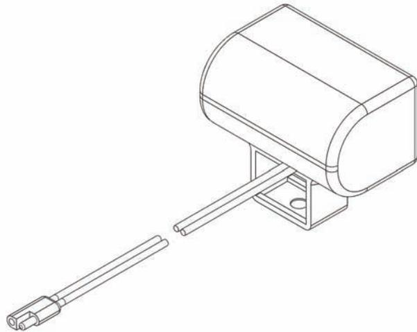
1. The best way for any wiring application is soldering each lead together and then covering each joint with shrink tubing.
