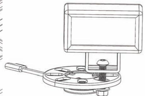
To mount lights to Power Pad place bolt through light bracket. Use one of the universal mounting slots on the Power Pad
