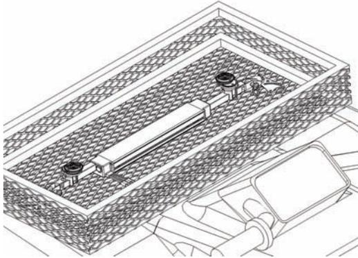
Place Power Rail into ATV basket. Place threaded mounting plates (12) under basket. Align holes in universal rail mounts (5) and threaded mounting plates (12) with holes in the metal mesh. Use provided bolts (11) and washers (9) to secure universal rail mounts (5).
