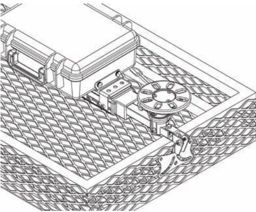
Center Power Rail on basket. Turn universal rail mounts (5) 90 degrees as shown.
