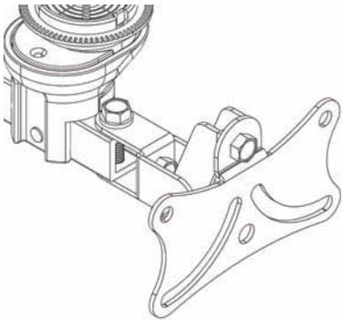
Rotate universal rail mounts (5) into the vertical position as shown.
