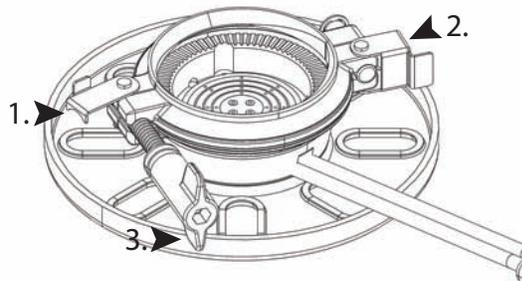
Unlatch nut (1) and clamp (2) locking tabs. Then unscrew wingnut (3).
