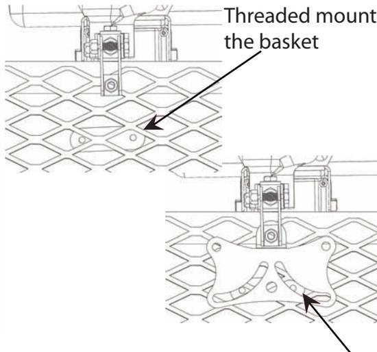
Align holes in universal rail mounts (5), expanded metal, and threaded mounting plate (12)
