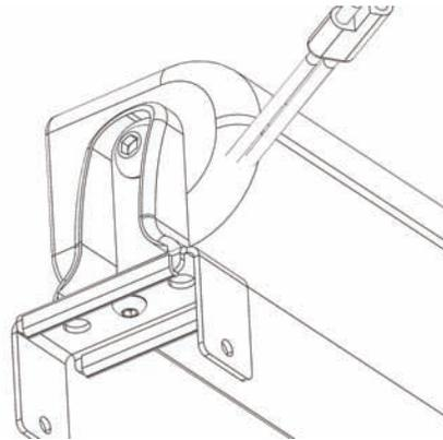
Mount middle accessory mounting brackets to OEM light mounts. Make sure to place bolt heads on the underside of the mounting brackets. This insures that the brackets will be able to lay flat on top of the Power Rail.
