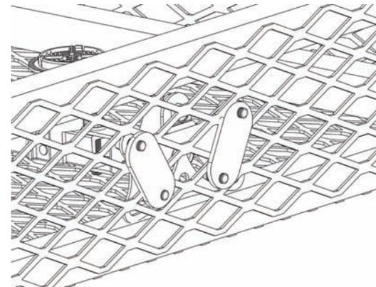
Place Power Rail into basket. Extend adjustable rail arms until universal rail mounts (5) are against side of basket. Then tighten arm locking screw. Thread provided bolts (11) and washers (9) into threaded mounting plates (12) as shown and tighten. Then repeat on the opposite side.
