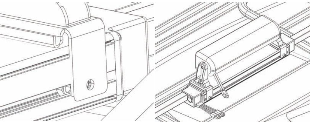
Center light with attached mounts on to the Power Rail. Move slide nuts until they are alined with mounting holes and tighten brackets using supplied thumb screws. Make sure to connect the LED light's power wire to black accessory power plug.
