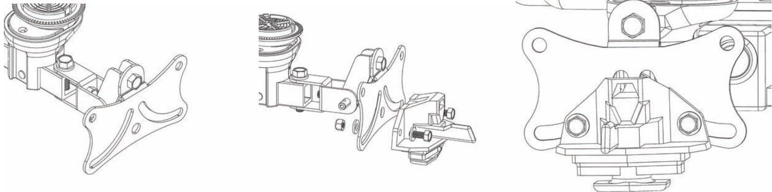
Rotate universal rail mounts (5) into the vertical position as shown.
