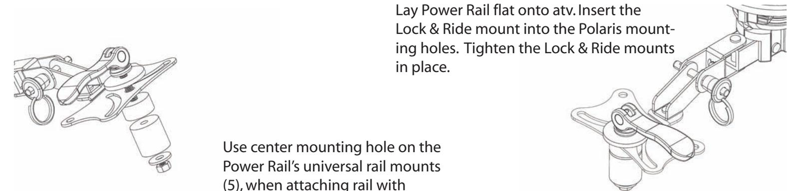
Lay Power Rail flat onto atv. Insert the Lock & Ride mount into the Polaris mounting holes. Tighten the Lock & Ride mounts in place.
