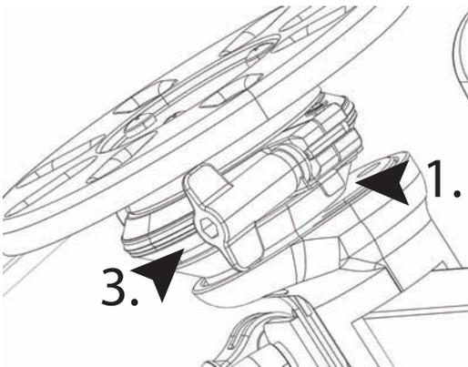
Tighten clamp wingnut (3). Then close nut locking tab (1).
